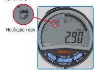
The calibration schedule warning icon starts blinking at a set time (e.g. 1 week before the calibration date) before the limit. If the limit is exceeded, the entire screen starts blinking to notify the user.
