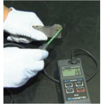
Measurement of residual magnetism
