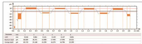
Example of SMD terminal height measurement by PFF
