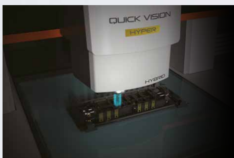
Example of measuring an engine control unit
