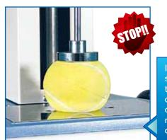
If the motorized stand goes beyond the overload value during its operation, it will not continue to operate.
