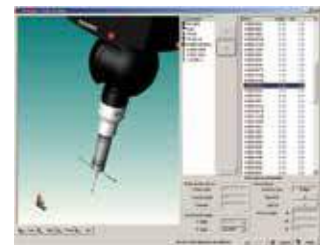
Example of sampling method: scanning measurement
