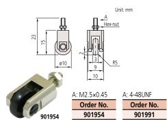
Roller material: Hardened steel Roller runout: 10 µm or better
