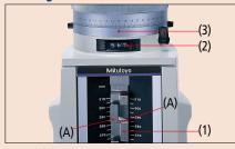
(A) Height A (1) Scale 280 mm (2) Counter 5.67 mm (3) Thimble 0.000 mm
