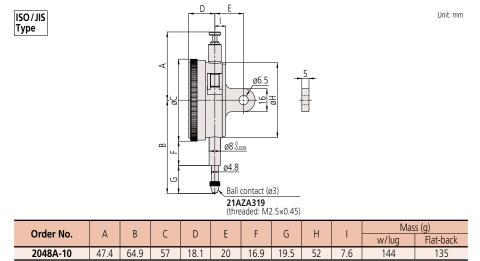
Note 1: Contact points, other than dedicated types, cannot be installed. Note 2: The shoulder on a contact point (standard accessory) acts as a stop to prevent spindle overrun that may otherwise damage the indicator. For this reason, if you need to install an optional contact point with an outside diameter smaller than 7 mm, use a washer (with outside diameter of at least 7 mm, inside diameter of 3 mm, and thickness of approx. 0.5 mm) placed between the contact point and the spindle.
