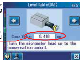
Amount of micrometer head adjustment required Leveling table (DAT) (Option)
